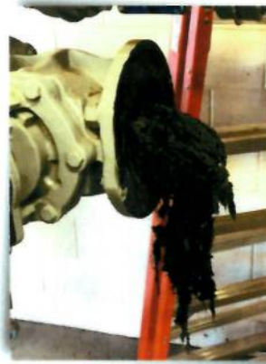
Wipes clog pipes (left) and equipment such as pumps (right), requiring regular, manual removal of wipes mixed with rags at Metro's Northern Treatment Plant (photo top of page).
