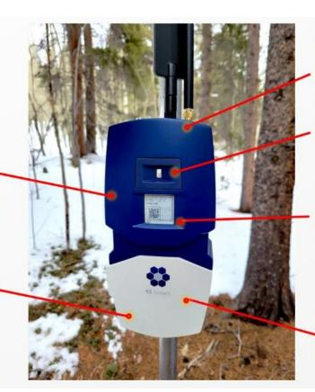
**Communication Capability** – LTE (Multicarrier/Worldwide) or LoRa. Satellite under development.
