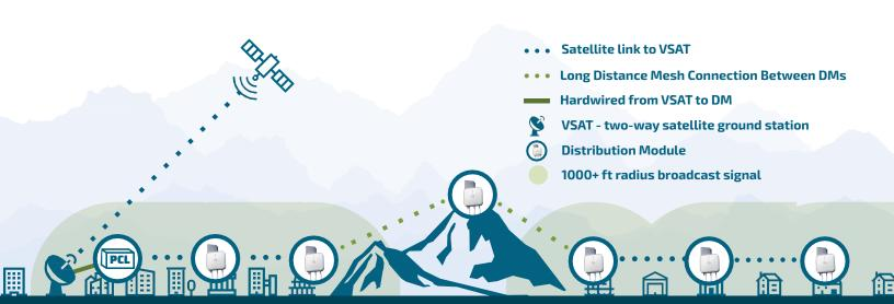
Portable Communications Link (PCL) creates a standalone network, aggregating the signal from existing satellite, ethernet, broadband or cellular networks.
