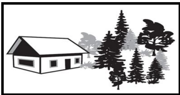
Figure 31 – Example of vegetation that is overgrown and has inadequate spacing between the home and vegetation.
