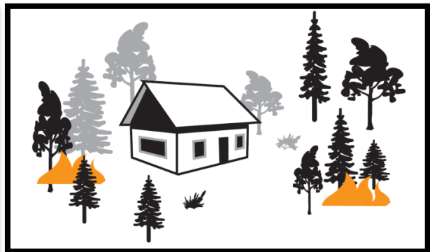
Figure 39 – Proper fuels management limits fire spread continuity and reduces the fire spread to the home.
