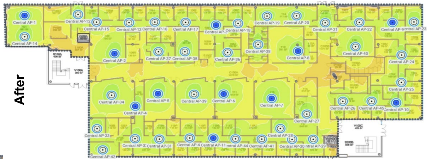
124 access points, comprehensive coverage
