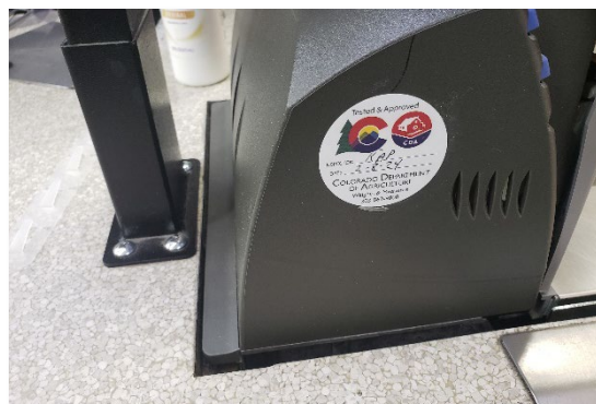
Inspectors with the Department of Agriculture's Division of Inspection and Consumer Services attach an approval sticker to licensed scales or other measuring devices that comply with NIST standards. Photo Credit: OSA Staff
