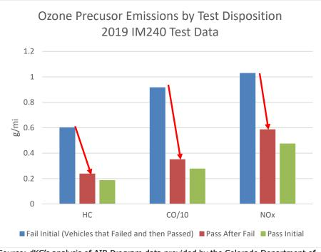
Exhibit 4. Ozone Precursor Emissions by Test Disposition, 2019 IM240 Test Data
